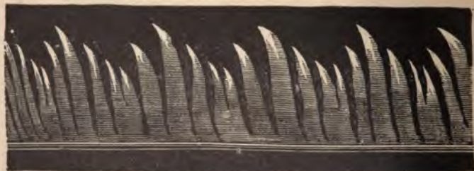
FIG. 14.—Manometric Flames produced by Koenig's apparatus. These illustrate a blending of two distinct musical notes.
